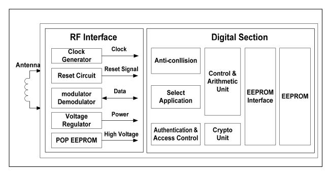
Figure 2-1 FM11RF32N Block Diagram
