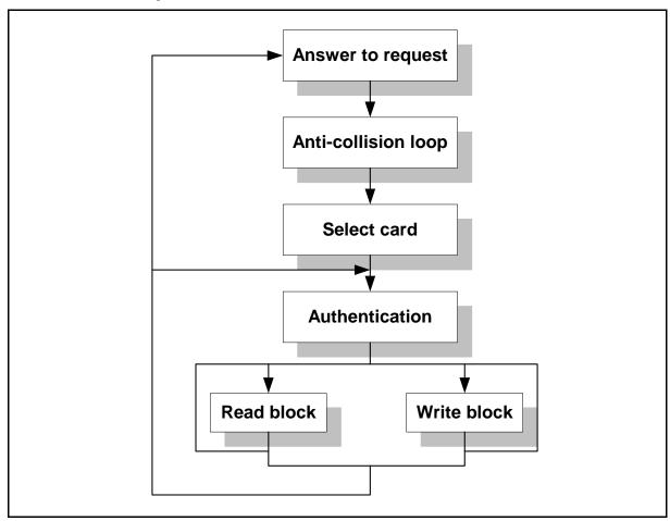
Figure 2-2 FM11RF32N Transaction sequence diagram
