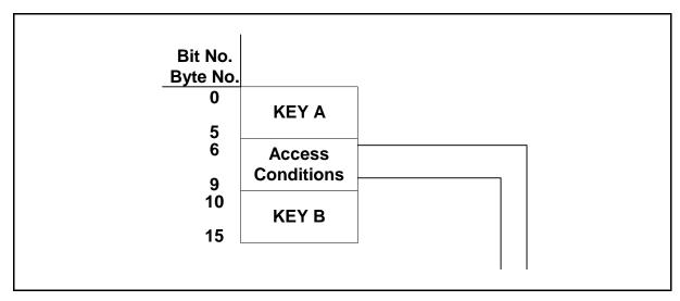
Figure 4-2 FM11RF32N Structure of the Control Block
